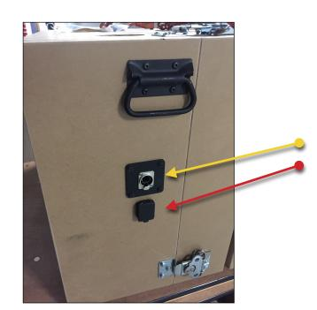
Locate external pass thru ports located on sides of each unit.
