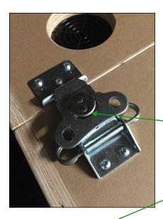
Separate horizontal finish box by unlatching 4 butterfly latches to access computers, plugins and motion sensor.
